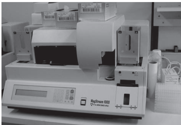
Figure 7. Instrument for automated measurement of haemoglobin concentration in faecal specimens.
